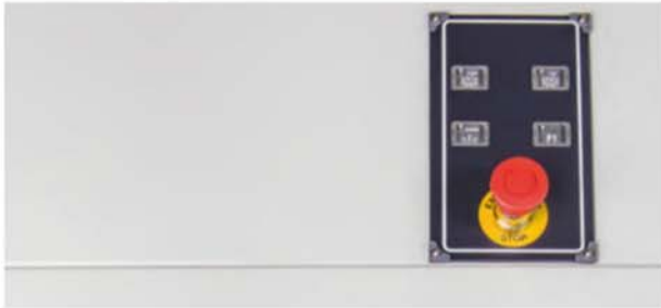
Emergency stop for operator's safety.
