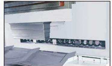
• Auger style chip conveyor makes chip disposal and collection easy; convenient.
