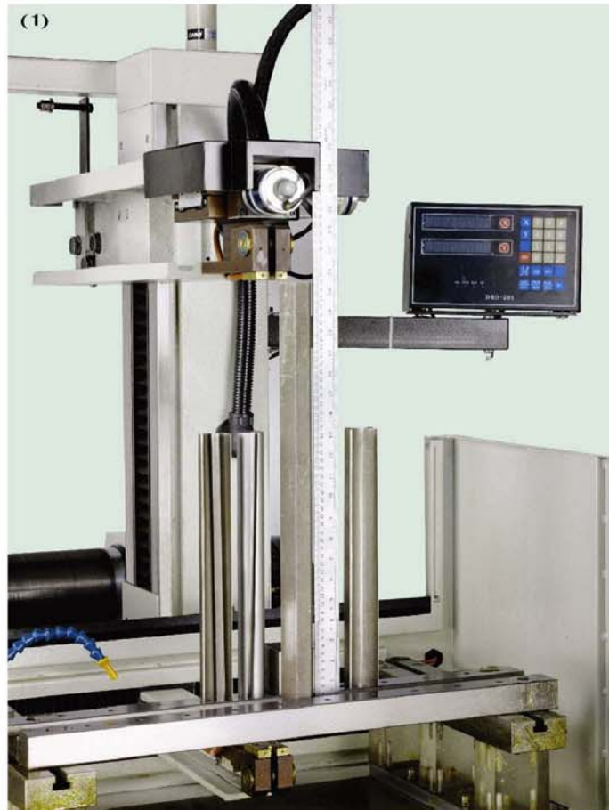
SIMPLE & ACCURACY. STANDARD MAXIMUM HIGH OF WORK-PIECE. 400mm. OPTIONAL : 600mm MAXIMUM.
